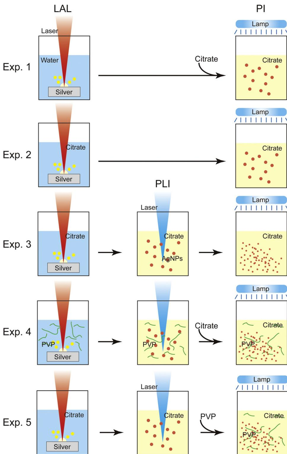
**Fig. 1.** Schematic diagrams of preparation procedure of the source silver colloids and photoirradiation. LAL, PLI, and PI stands for laser ablation in liquids for preparation of silver NPs, post laser irradiation to reduce particle size, and photoirradiation to induce the shape conversion. The experimental conditions are shown in text. The order of adding of citrate and PVP was different among the experiments.
